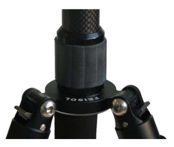
For additional extension (CT-3441S and CT-3441SB only) there is a telescopable second Center Column Section which can be released by turning the top twistlock located just below the top of the lower Center Column Section (see picture) a half turn in counterclockwise direction, extending, and securely re-locking the twistlock. Please do not over-tighten.
