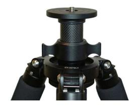
To make Leveling adjustments, please unlock the twistlock located just below the mainframe (see picture) by turning it half a turn in counterclockwise direction. Once the lock is released, the axis of the Center Column can be moved to level. After setting the column at the desired angle, turn the twistlock in clockwise direction to securely lock the column into place. Please do not over-tighten.
