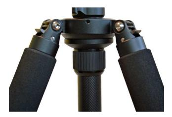
To remove the Leveling Column (in order to install a flat Ball-Head mount/ Center Column mount/ Leveling Base), unscrew the plate at the bottom of the Center Column by turning it counterclockwise (see picture).
