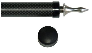
Model CM-1471: Remove the rubber cap at the end of the leg by inserting a wooden stick or similar object between the rubber cap and the aluminum ring at the end of the leg (see picture). By pushing forward around the ring, the rubber cap can be removed, exposing a thread into which the spike can be screwed and locked tightly into place with the included wrench.
